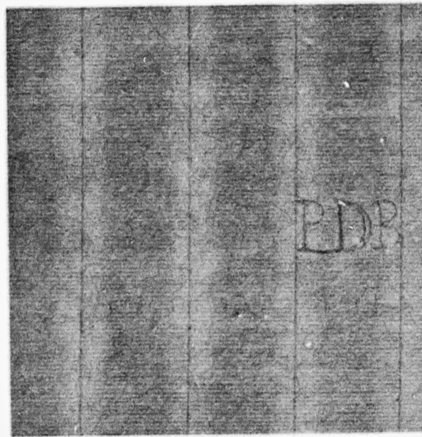
Beta radiograph of 0.16 mm thick paper sample, following the acquisition setup detailed in the diagram above, with an exposure time of 15 minutes, and scanned at “Low IPI”
