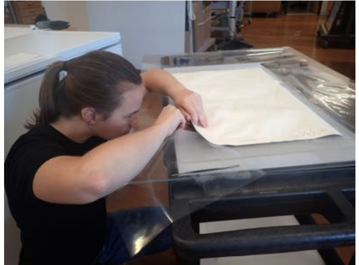
Figure 4: Popping the frozen ink from the acrylic with a microspatula.
