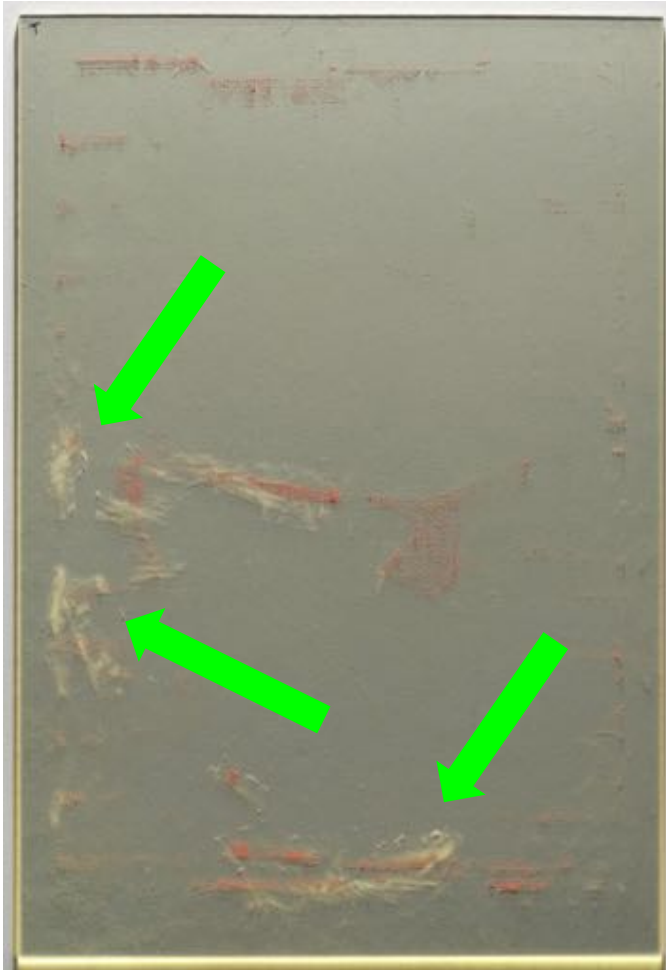
Figure 6: The acrylic after removal, raking light. Red stains are visible, as are scratches left by the blade, indicated by the green arrows.
