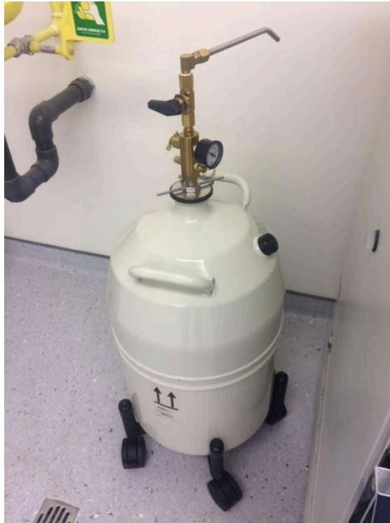
MVE Lab 20 Liquid Nitrogen dewar on casters with manual liquid discharge device installed
