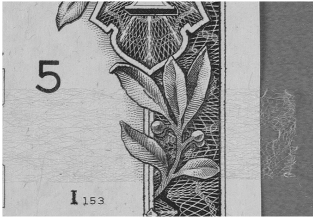
Fig. 1. Strip of 1.6g tissue precoated with 5% Klucel G on a dollar bill. Note hole in tissue caused by tweezers at the edge.
