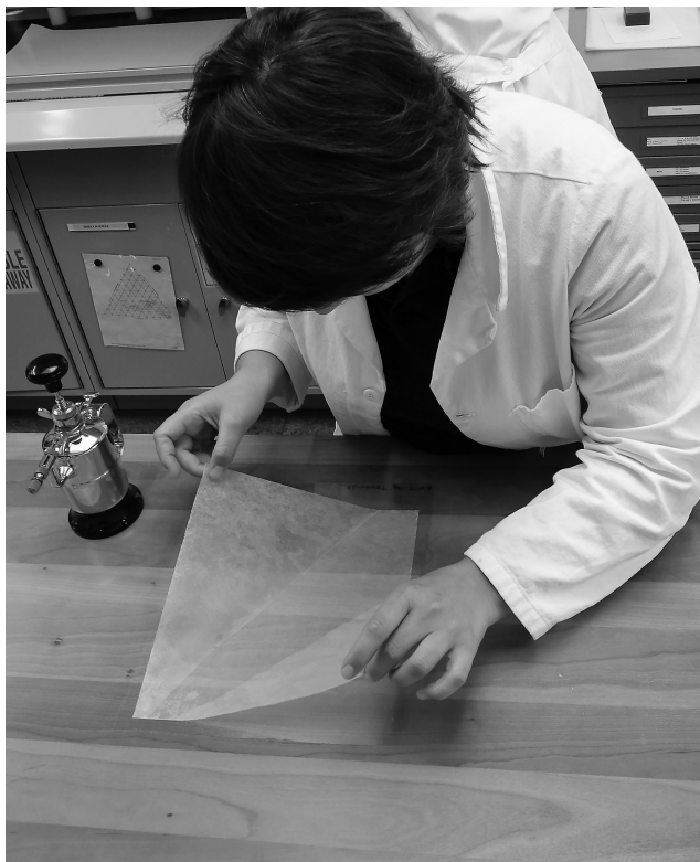
Fig. 2. A liberal spray of water on the adhesive coating just prior to dropping the tissue minimizes the chance of wrinkles.
