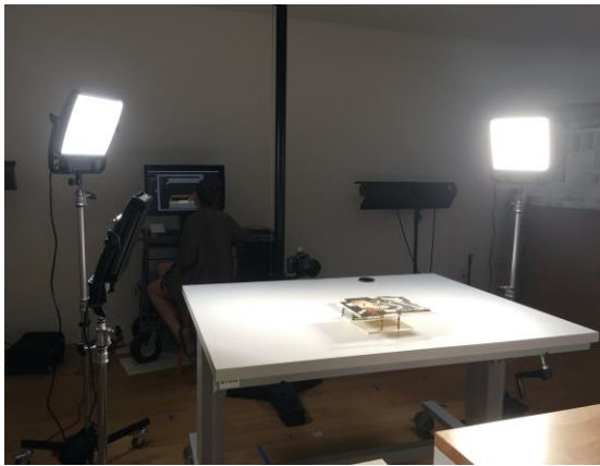
Fig. 1. Imaging of a Minotaure periodical before treatment. Shown in use are three LED Litepanels lights with diffusing gel or honeycomb grid filters. All lights are being controlled by an iPad with SLD app. Image courtesy of Ashley Stanford.
