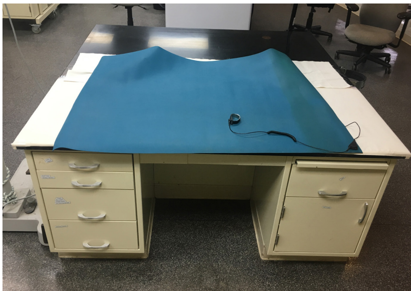
Figure 1. Left: Electrostatic discharge mat on workbench ready for ordnance. Above: Metal bracelet worn in conjunction with an electrostatic discharge mat to ground the user. All images courtesy the Virginia Department of Historic Resources.
