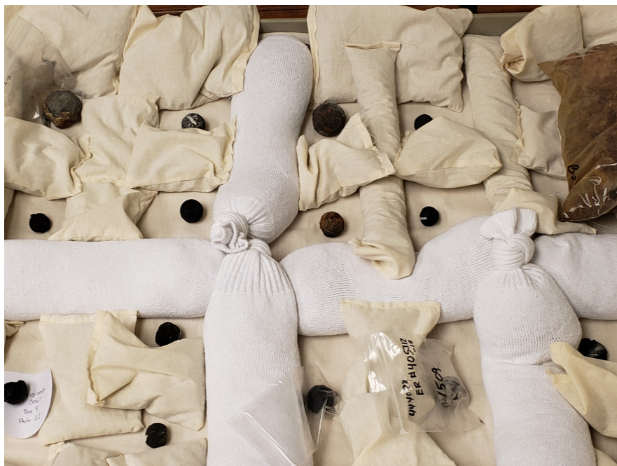
Figure 3. Cart prepared with materials to prevent static and impact while transporting possible live ordnance.
