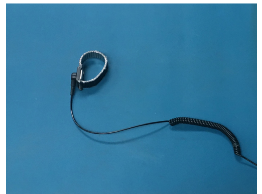
Figure 1. Left: Electrostatic discharge mat on workbench ready for ordnance. Above: Metal bracelet worn in conjunction with an electrostatic discharge mat to ground the user. All images courtesy the Virginia Department of Historic Resources.
