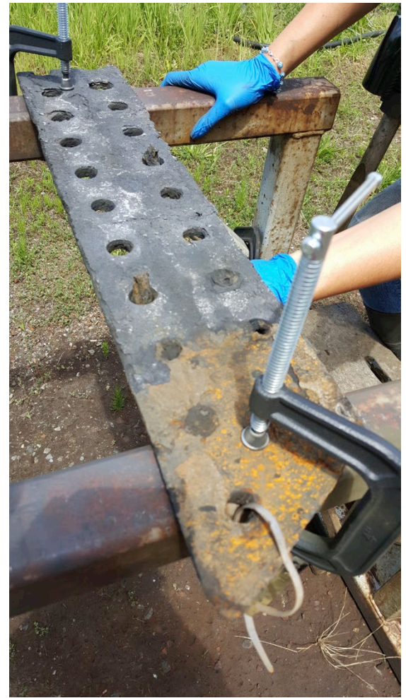
Figure 2. An archaeological iron object is held in place using two clamps and attaching the object to saw-horses, so that the object does not move during dry ice blasting. Image courtesy of The Mariners' Museum and Park.
