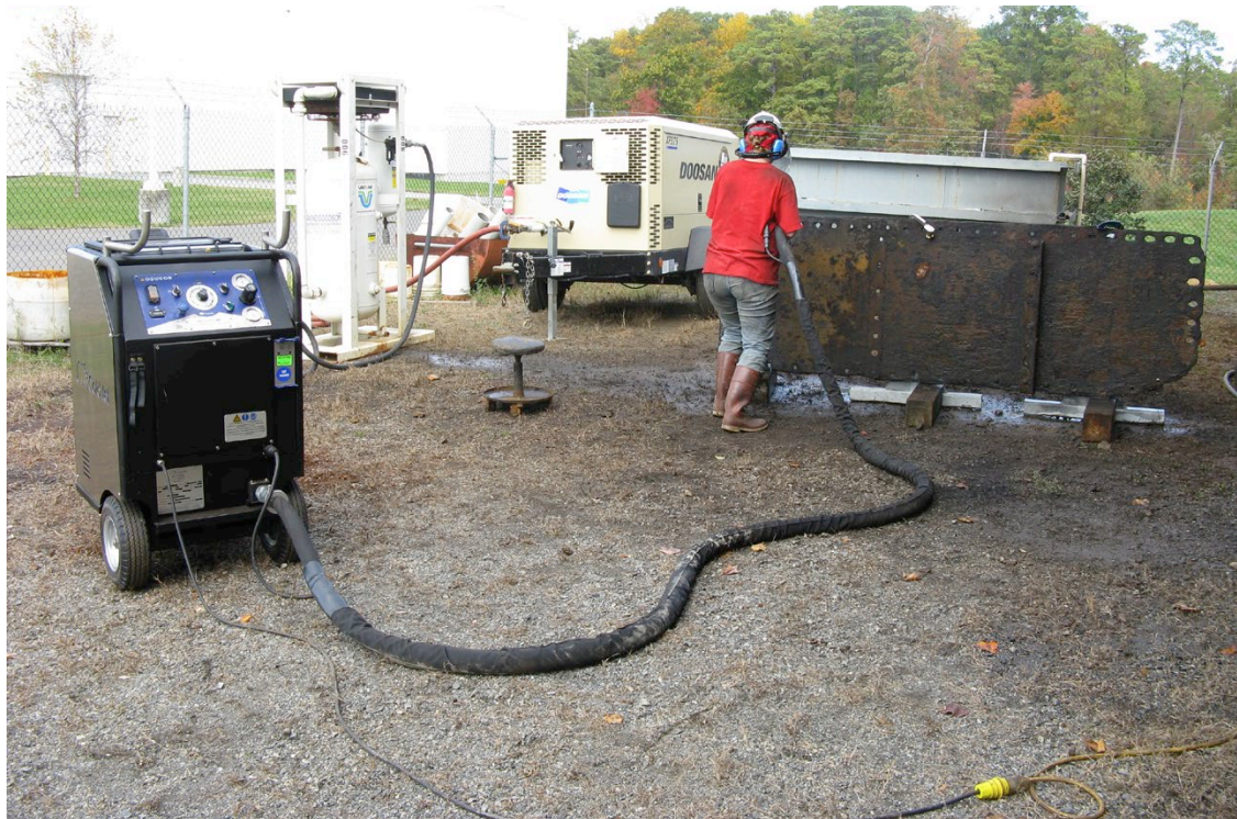
Figure 1. Mariners' staff member Kate Sullivan is seen treating an archaeological iron object, with DIB unit (left), the air dryer (middle), and air compressor (right). Image courtesy of The Mariners' Museum and Park.
