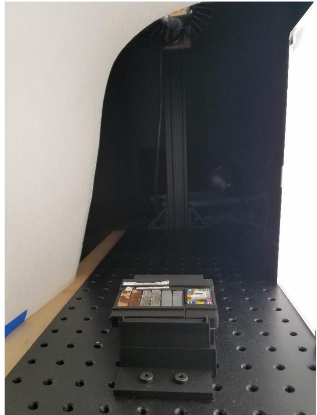
Figure 24: image of the photo stand from in front of the camera with side angle lighting
