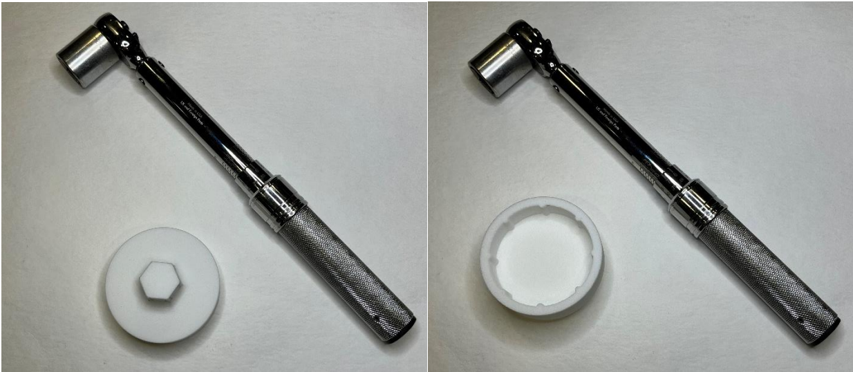
Figures 11 & 12: 3D printed torque wrench socket produced to fit GL45 cap and CDI 1502MRMH-QR torque wrench (2.8-16.4 Nm range) used for tightening lids consistently.
