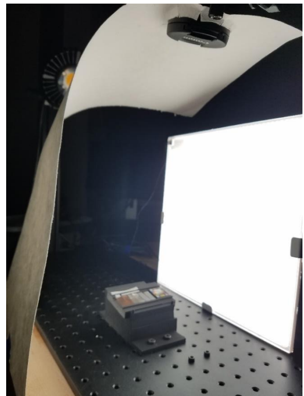
Figure 26: image of the photo stand from the left side of the camera with side angle lighting
