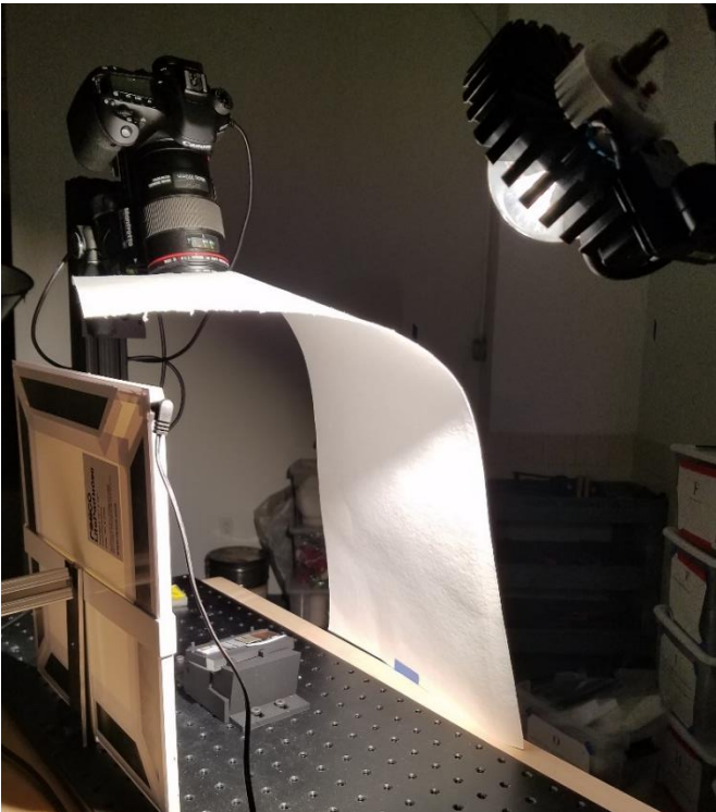
Figure 30: image of the photo stand from the left of the glancing angle light with the light on
