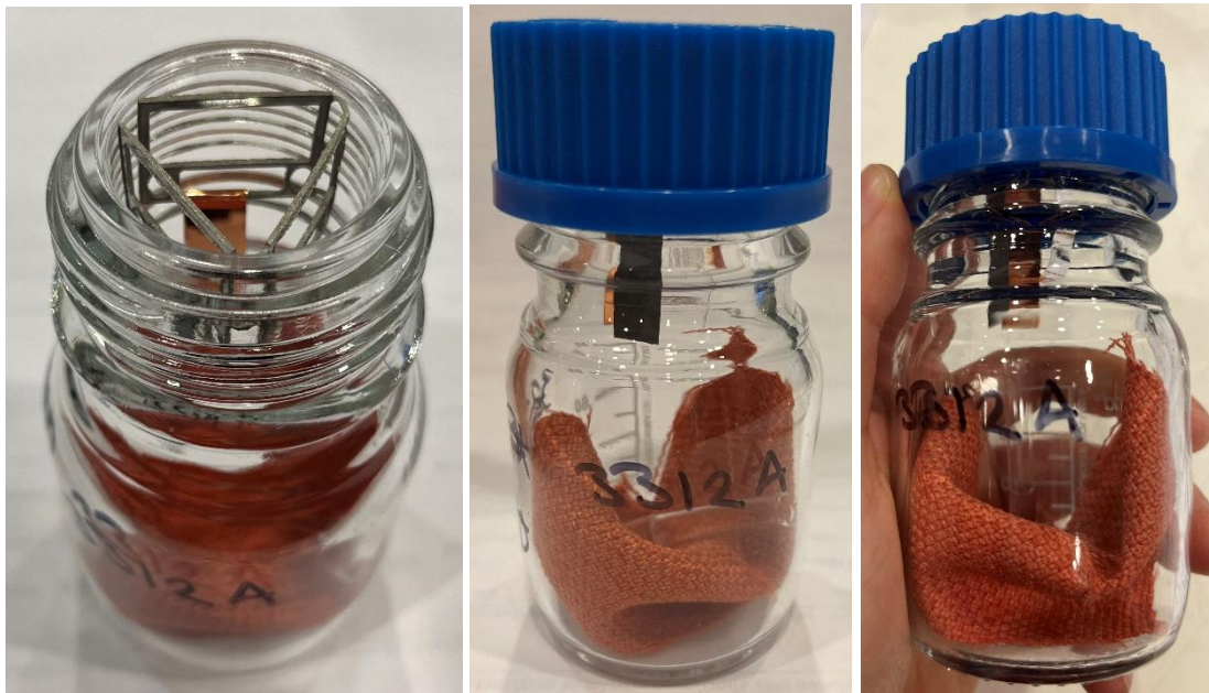
Figures 8, 9 & 10: Left: a coupon holder placed in the neck of a sample jar. Center and Right: A sealed sample jar with hanger, coupons, test material, water and vial.
