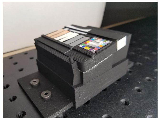
Figure 20: image of the coupon stage bolted down on the photo stand. The stage is in between the Rosco LitePad LED and the paper board used to diffuse the lighting.
