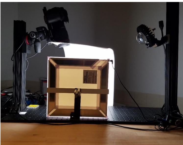
Figures 21 & 22 : Left: image of the photo stand with only the diffuse light illuminated. Right: image of the photo stand with only the glancing-angle light illuminated.
