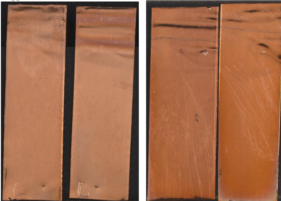
Figures 13 & 14: Left: acceptable amount of minimal corrosion for control. Right: too much corrosion, observed as darkening, for control.
