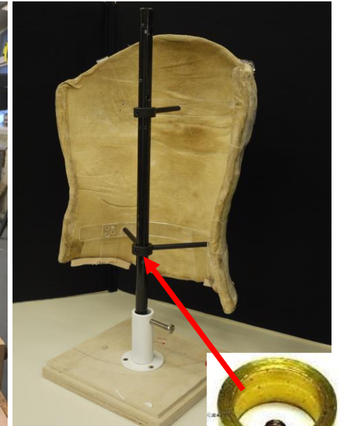
Adjustable steel collars fastened onto vertical pole
