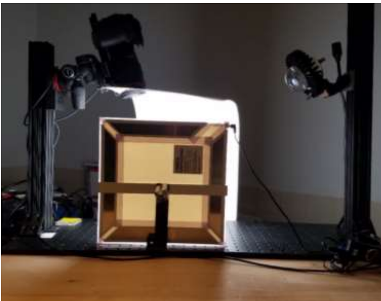
Figures 17 (left) & 18 (right): Left: image of the photo stand with only the diffuse light illuminated. Right: image of the photo stand with only the glancing-angle light illuminated.
