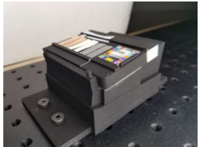
Figure 16: image of the coupon stage bolted down on the photo stand. The stage is in between the Rosco LitePad LED and the paper board used to diffuse the lighting.
