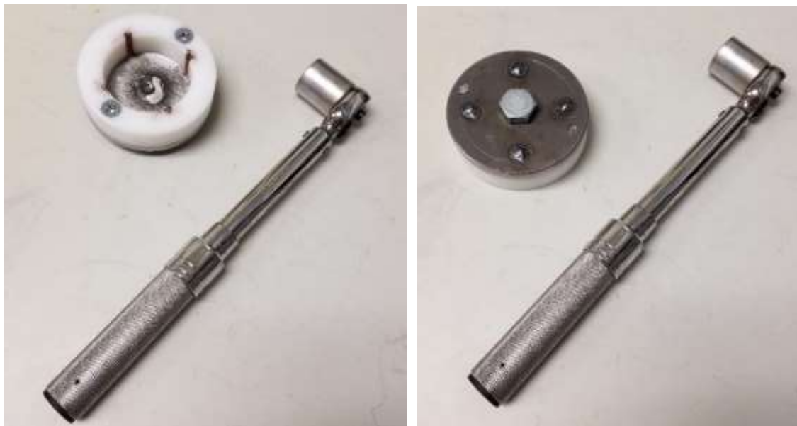
Figure 7 & 8: Custom torque wrench socket produced to fit GL45 cap and CDI 1502MRMH-QR torque wrench (2.8-16.4 Nm range) used for tightening lids consistently.
