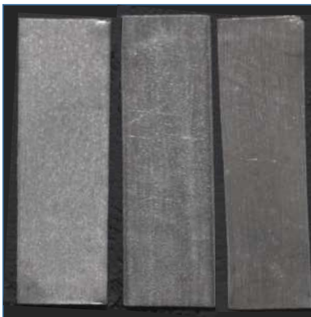
Figure 2: Left: a properly sanded lead coupon. Middle: a partially over-sanded lead coupon. Right: a fully over-sanded shiny lead coupon.
