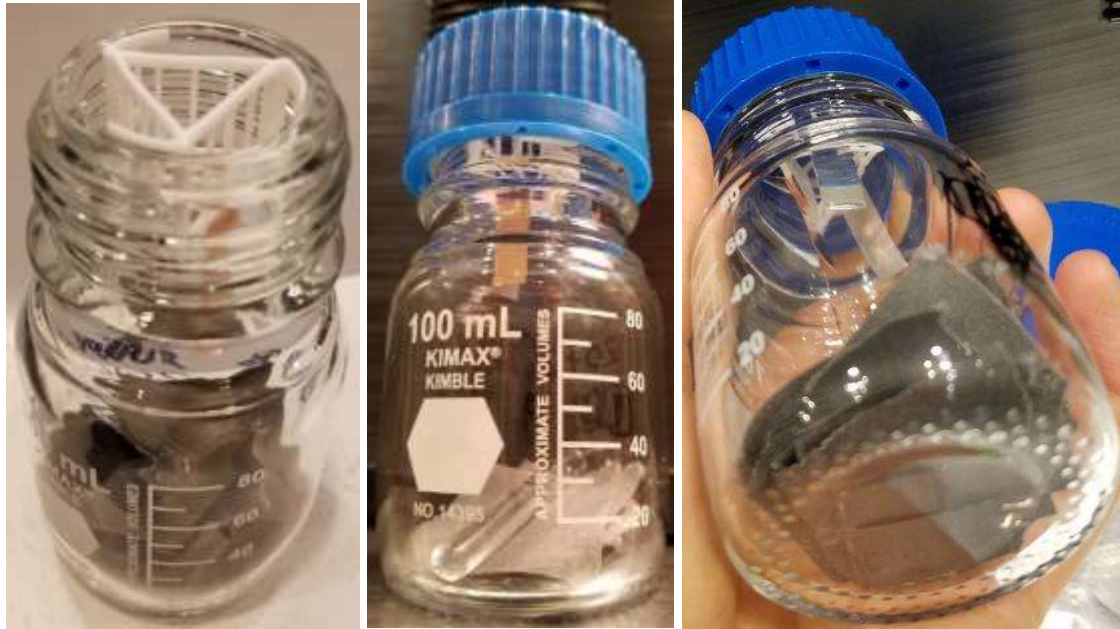
Figure 6: Left: a coupon holder placed in the neck of a sample jar. Center and Right: A sealed sample jar with hanger, coupons, test material, water and vial.
