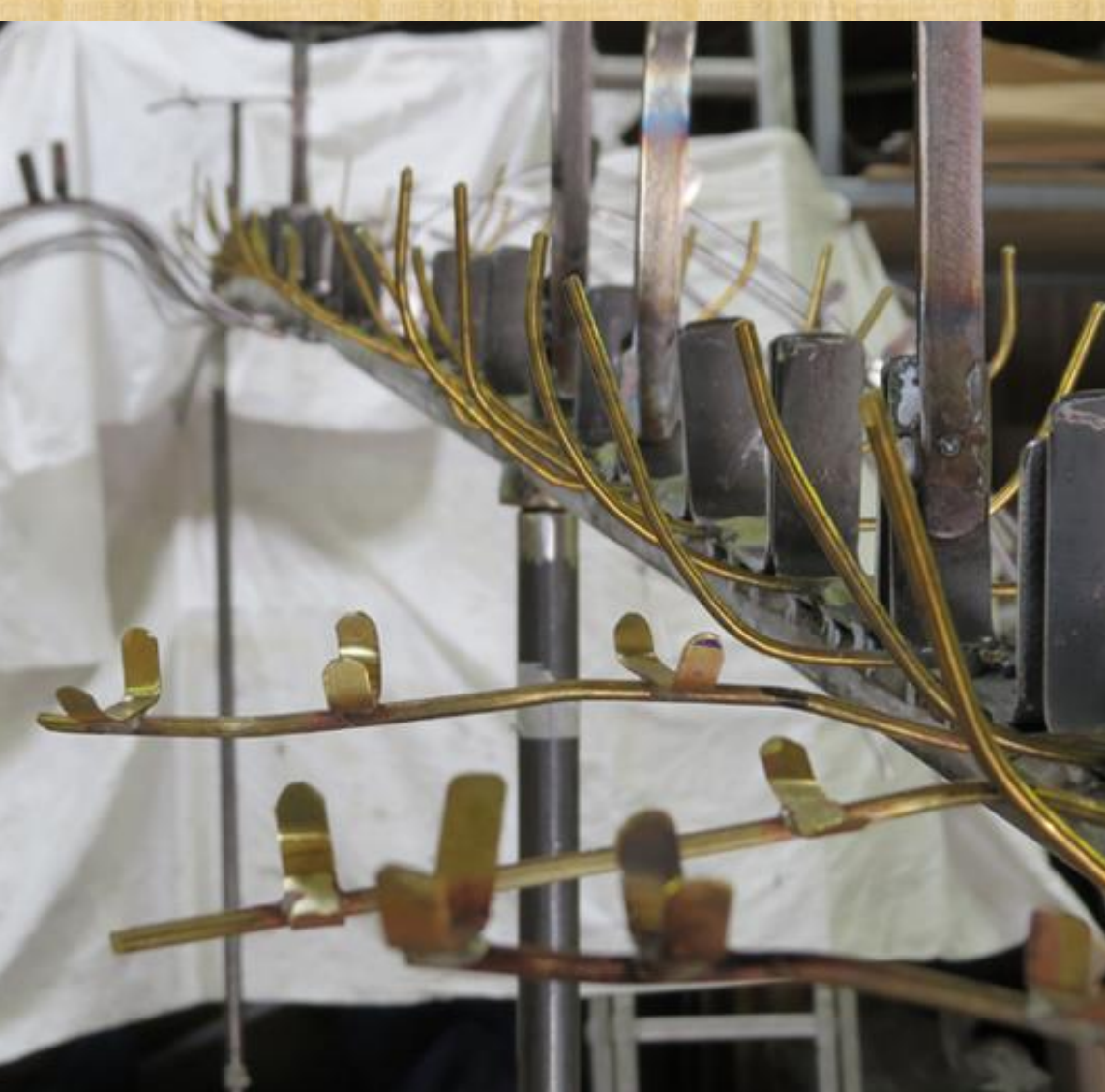
Figure 4. Brass strips and rods brazed together to hold smaller bones in place.
