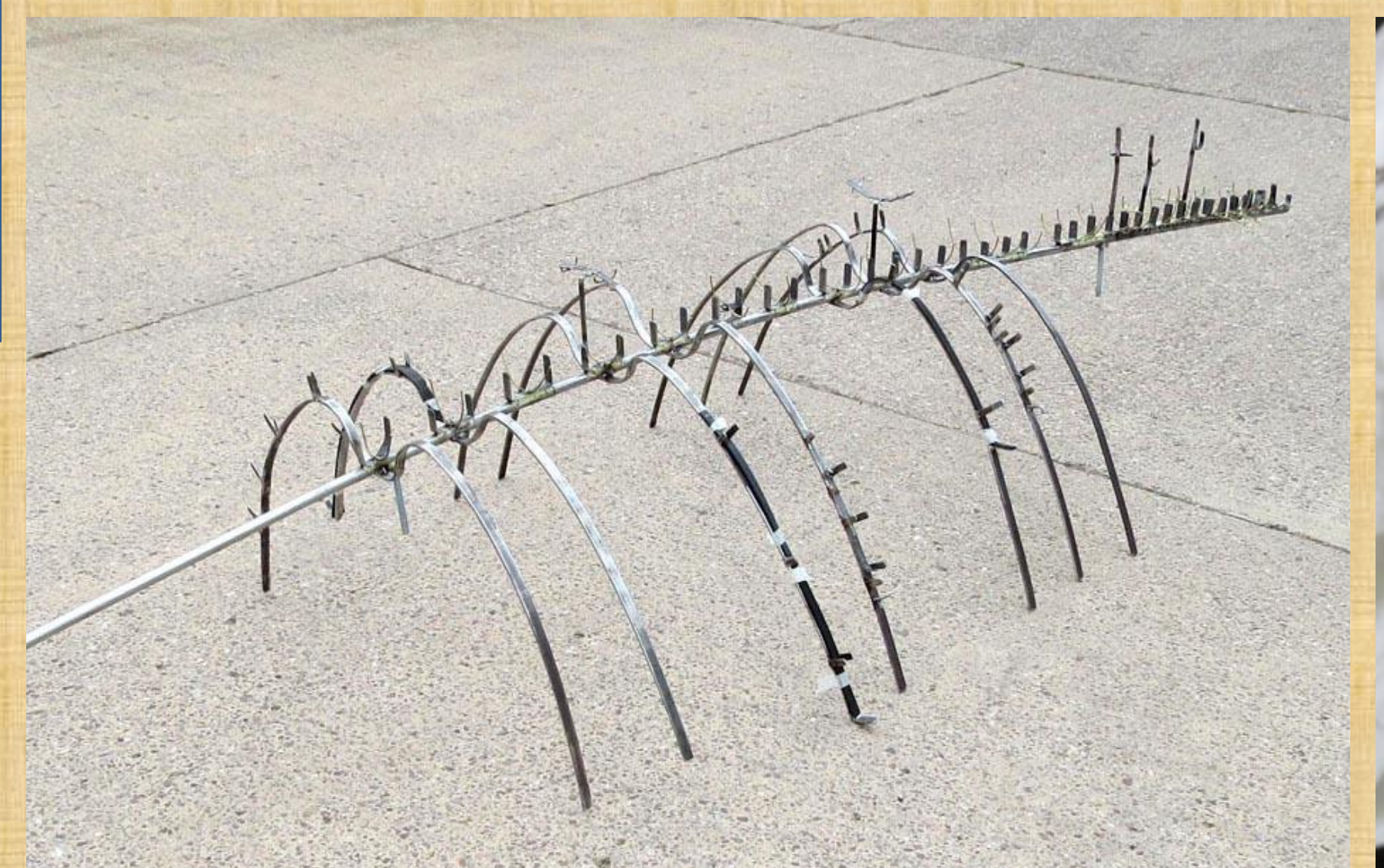
Figure 3. The steel frame made to hold the larger ribs and vertebrae in place, not yet positioned on the upright supports.
