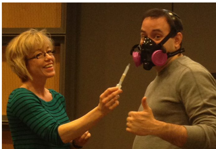
Industrial hygienist Lee Foley conducts a respirator fit test for conservator Steven Pickman at a Washington Conservation Guild fit test. Photo courtesy of Anne Kingery-Schwartz.
