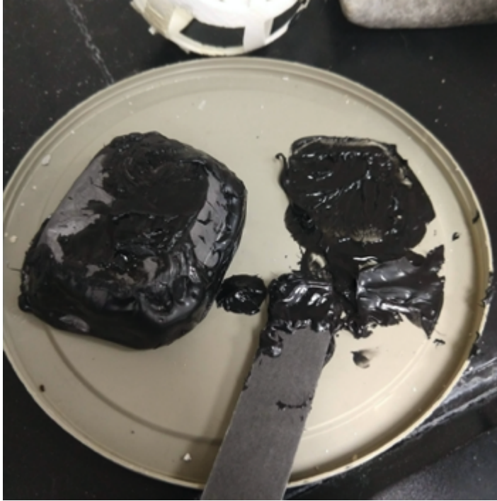
Fig. 6. Plasti Dip smeared over lead weight and scrap barrier board.
