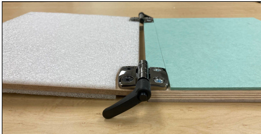
The upper board (left) is filled using lightweight materials; the lower board (right) is filled using heavy materials.
