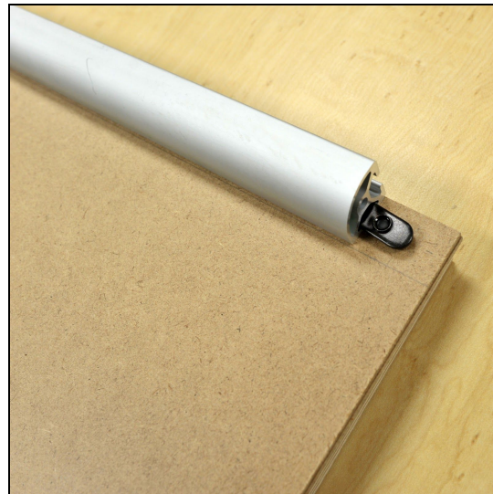
Sliding the T-slotted framing onto the 1/4-20 nuts.
