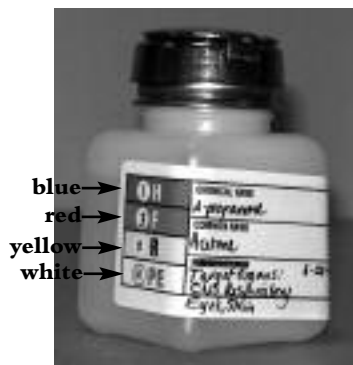
Figure 8. A properly labeled hazardous chemical container.
