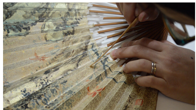
Fig. 7. Once the paper strip and carrier could not be pushed any further, use the bamboo spatula's tip to push paper in more.
