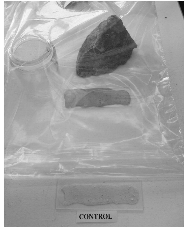
Cinnabar ore with mercury -indicating powder slide inside a bag with control slide on the outside of the bag after two weeks. [Image: Donna Strahan/Taylor & Francis]
