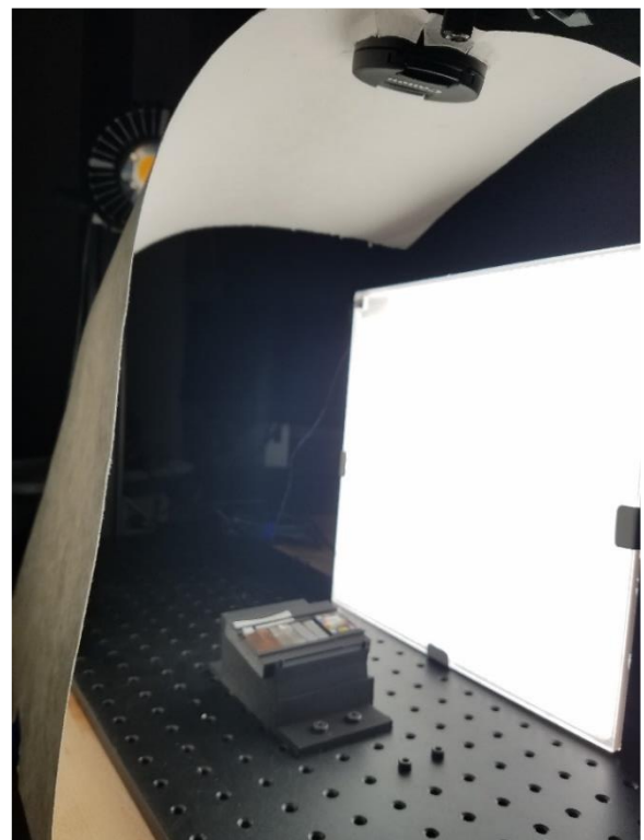
Figure 35: image of the photo stand from the left side of the camera with side angle lighting
