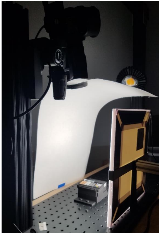
Figure 34: image of the photo stand from the right side of the camera with side angle lighting
