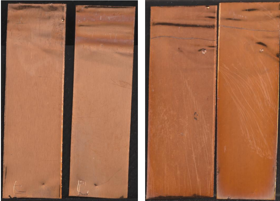
Figures 24 & 25 Left: acceptable amount of minimal corrosion for control. Right: too much corrosion, observed as reddening, for control.
