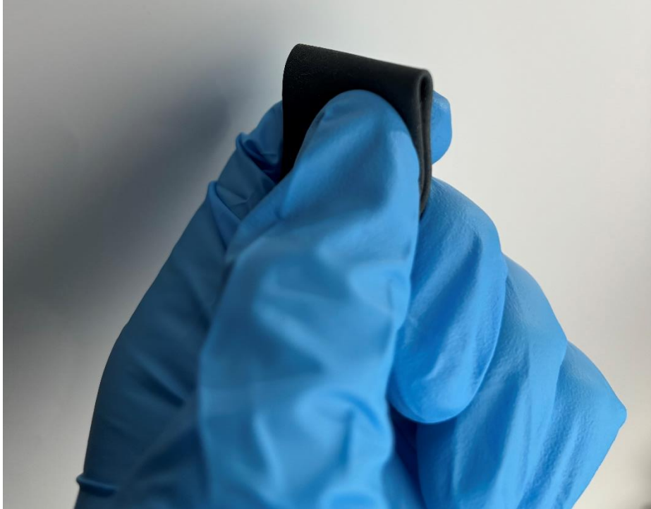
Figure 2: how to properly fold and hold the sandpaper. Thumb and forefinger as close to the fold as possible without touching the lead during sanding.
