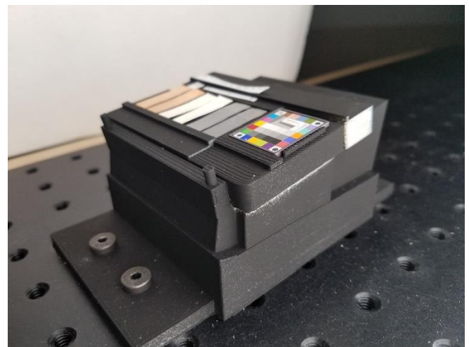
Figure 29: image of the coupon stage bolted down on the photo stand. The stage is in between the Rosco LitePad LED and the paper board used to diffuse the lighting.
