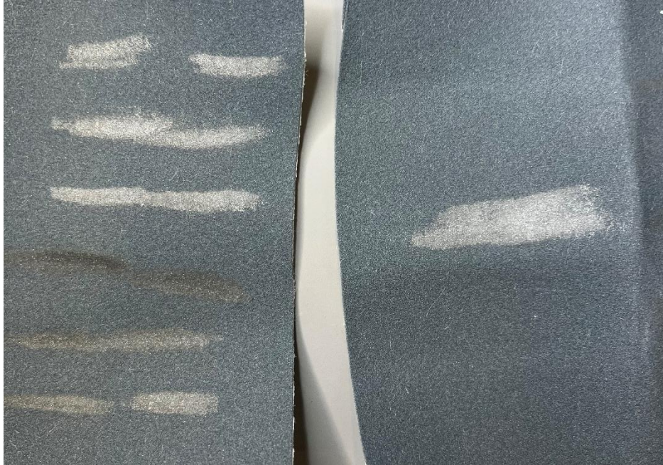
Figure 4: Left: lead residue on sandpaper after using proper sanding technique. Each mark represents ~10-15 strokes of sanding, one on the left and right in 6 different locations on the sandpaper. A correct, small/thin surface area in contact with the lead coupon is shown. Right: lead residue after improper sanding technique. Too large of a surface area in contact with the lead coupon.
