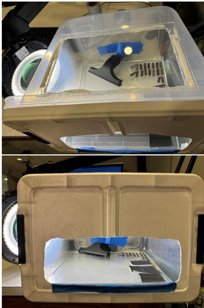
Figures 5 & 6: Top: Top view of filtration box with glass top for viewing and glancing angle light to the left. Bottom: Front view of the filtration box, showing the filtered vacuum that pulls air from the back of the box.
