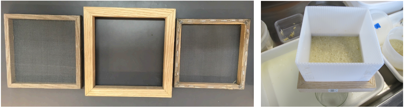
Figure 1: Boardmaking form with primary mould (left) deckle (center) and secondary mould (right); and form fitted with extend deckle made with coroplast.
