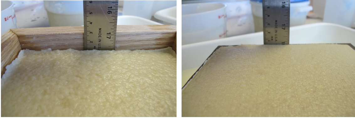
Figure 3 Sheet before and after the second mould is inserted, which reduces the thickness of the sheet
