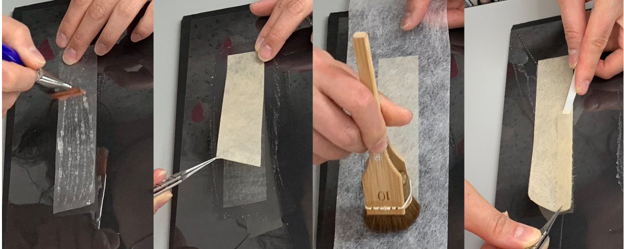
Fig. 3. From left to right: gluing up Goldbeater's skin, attaching toned Hollytex, smoothing down, and attaching glued-up strips of toned Tengujo paper.
