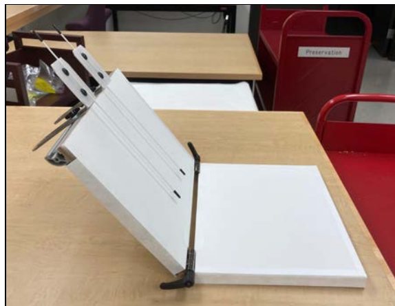
When properly weighted with covering materials, the ACBS should be balanced at obtuse angles.
