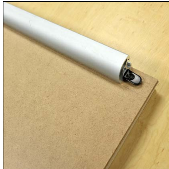
Sliding the T-slotted framing onto the ¼-20 nuts.
