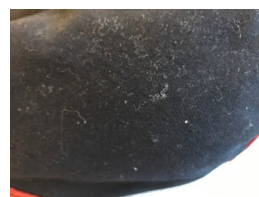
Figure 5: Polyester fibers attached to wool fabric of a military uniform.
