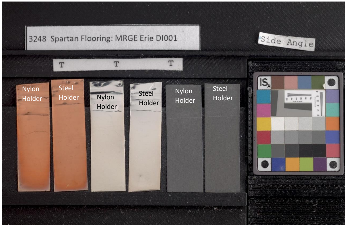
Figure 4: Coupons from Oddy test of MRGE Erie DI001 vinyl flooring. In each pair of coupons, those from the jar with the nylon holder are on the left, and the steel holder are on the right. No significant differences were observed between coupons from different jars.
