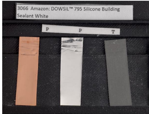
Figure 12: Coupons from a test of Dowsil™ 795 in jars with nylon holders (left) and in the jar with a steel holder (right).
