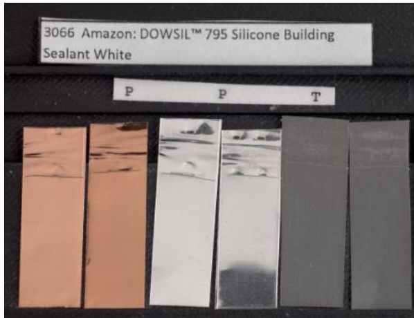
Figure 12: Coupons from a test of Dowsil™ 795 in jars with nylon holders (left) and in the jar with a steel holder (right).
