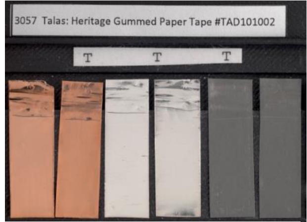
Figure 8: Coupons from jars with nylon holders and the temporary standard (left) and coupons from jars with steel holders and the temporary standard (right). Very slight yellow tarnish is visible around the edges of the nylon holder silvers, whereas the steel holder silvers were marked “T” for slight white haze which is not caused by tarnishing.
