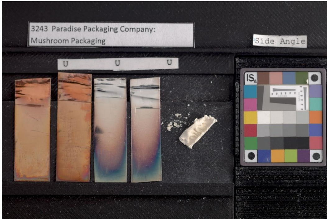
Figure 19: Coupons from a test of Paradise Packaging Company Mushroom Packaging. For each metal type, the coupons from the jar with the nylon holder are on the left, and the steel holder are on the right. The silver coupons were rated Unsuitable for extreme rainbow and purple tarnish overall.
