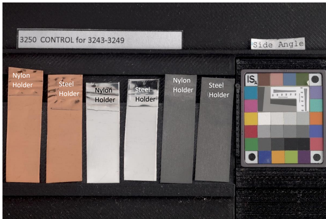
Figure 14: Coupons from a control test. In each pair of coupons, those from the jar with the nylon holder are on the left, and the steel holder are on the right.
