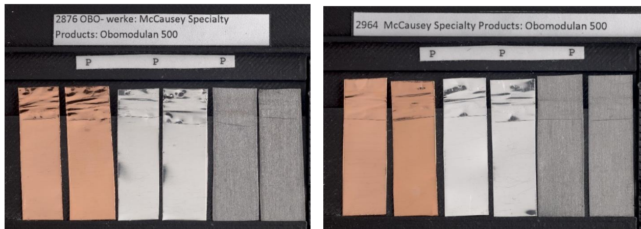
Figure 7: Coupons from jars with nylon holders and the permanent standard (left) and coupons from jars with steel holders and the permanent standard (right).
