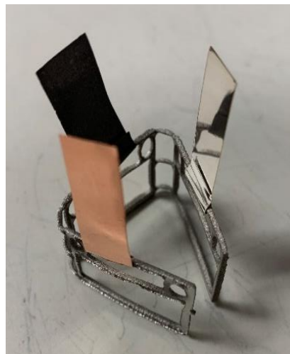
Figure 1: Stainless steel coupon holder with attached copper, silver, and lead coupons.
