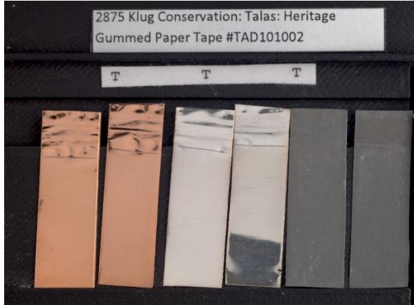
Figure 8: Coupons from jars with nylon holders and the temporary standard (left) and coupons from jars with steel holders and the temporary standard (right). Very slight yellow tarnish is visible around the edges of the nylon holder silvers, whereas the steel holder silvers were marked “T” for slight white haze which is not caused by tarnishing.
