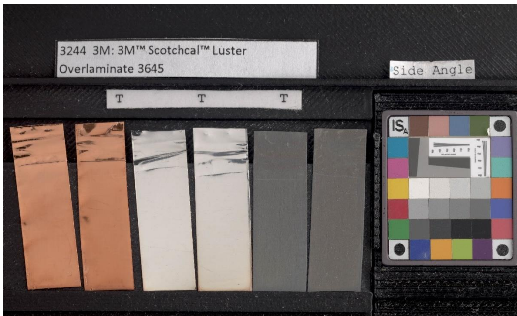
Figure 18: Coupons from a control test. For each metal type, the coupons from the jar with the nylon holder are on the left, and the steel holder are on the right. The silver coupons were rated T for slight yellow tarnish at the edges.
