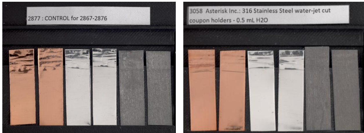
Figure 6: Control coupons from jars with nylon holders (left) and control coupons from jars with steel holders (right).
