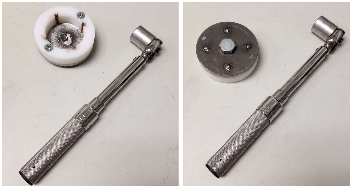
Figure 6 & 7: Custom torque wrench socket produced to fit GL45 cap and CDI 1502MRMH-QR torque wrench (2.8-16.4 Nm range) used for tightening lids consistently.
