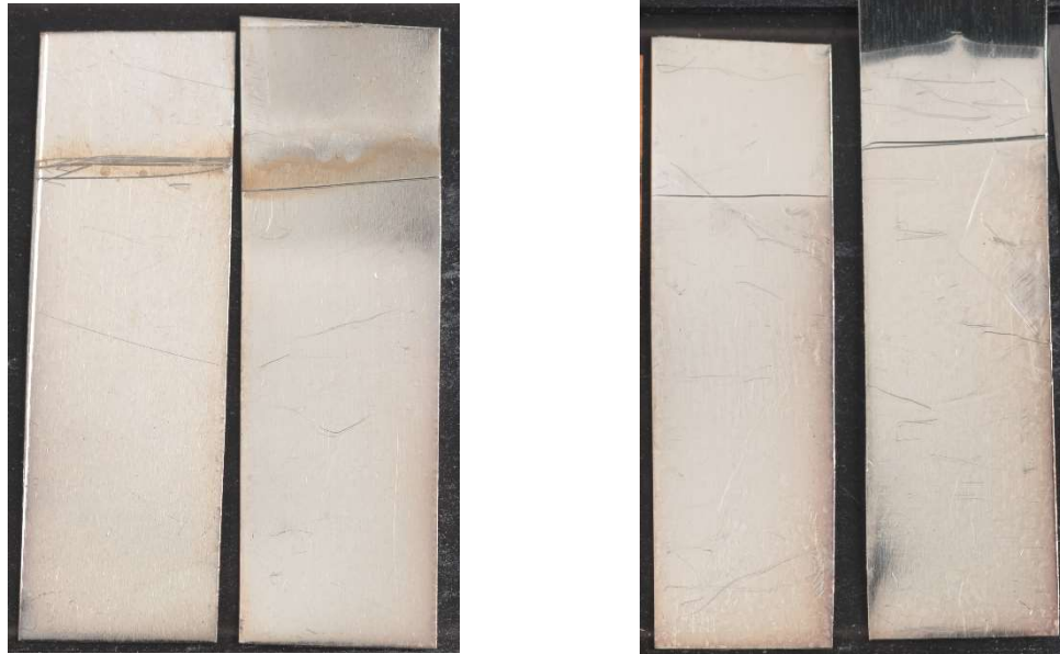
Figure 10 & 11: Left: acceptable amount of minimal corrosion for control. Right: too much corrosion for control.
