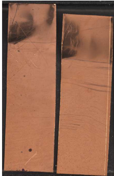
Figure 9 & 10: Left: acceptable amount of minimal corrosion for control. Right: too much corrosion for control.
