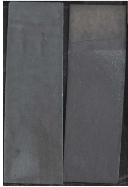
Figure 8 & 9: Left: acceptable amount of minimal corrosion for control. Right: too much corrosion for control.
