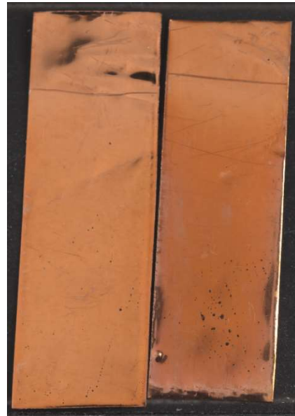
Figure 9 & 10: Left: acceptable amount of minimal corrosion for control. Right: too much corrosion for control.
