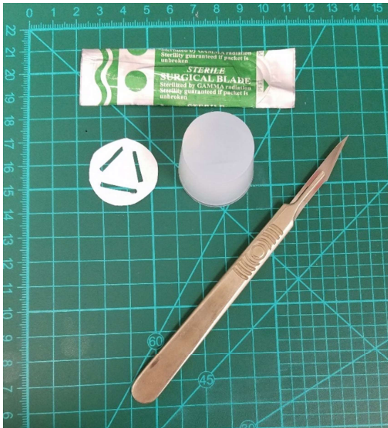
Figure 3: Left: The template and scalpel used for incising the stopper. Right: actual size of the template.
