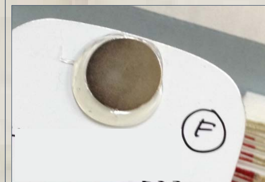
Upper Left: 1" diameter x 1/16" thick N42 Neodymium rare-earth magnets are attached to the front of 1/8" Dibond sheet insert using 3M 3792 low melt hot glue when the glue cools enough to be liquid but only warm to touch.
