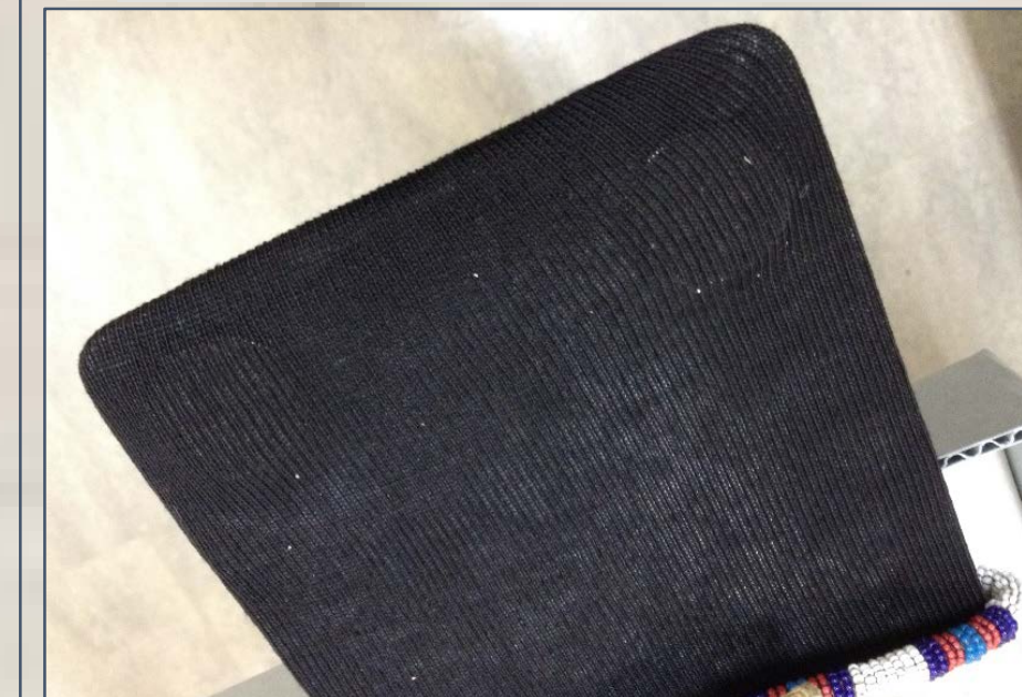
Lower Left: The edges of the Dibond insert are filed smooth, then covered with a layer of 1/8" polyester batting topped with black stockinette with the ribs aligned vertically to make it easier to slide the insert in and out of the bag.
